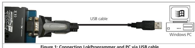
Figure 1: Connection LokProgrammer and PC via USB cable
